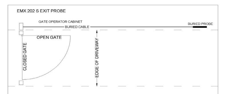
The EMX 202 S probe is used to open the gate for vehicles leaving the property. Bury the probe as far back from the gate as the cable will allow. Six to eight inches is deep enough for the probe and the cable. Connect the color-coded cable wires to the gate operator as shown below.
